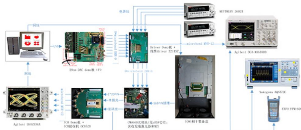
*High-speed optical communication environment based on Simulink. It integrates high-speed optical transceivers and modules, which can verify the whole system algorithm by oscilloscope.*
