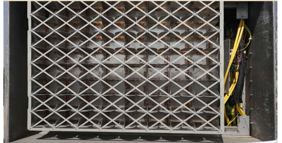
144 Element Vivaldi Antenna Array
