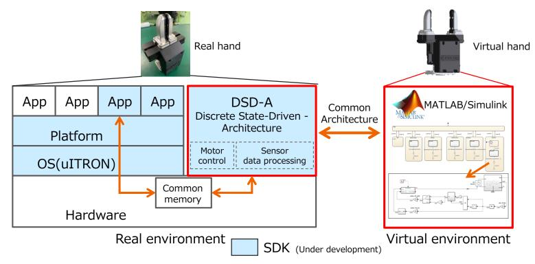
By using our proposed SDK, we believe that we will be able to develop this robot hand systems efficiently and respond quickly to diverse customer demands.
