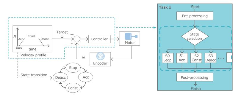
+ The program is divided for each possible state of the actuators and sensor. Also, as the status transition from one to another periodically, the processing time of the program can be controlled, thus real-time processing can be assured.
