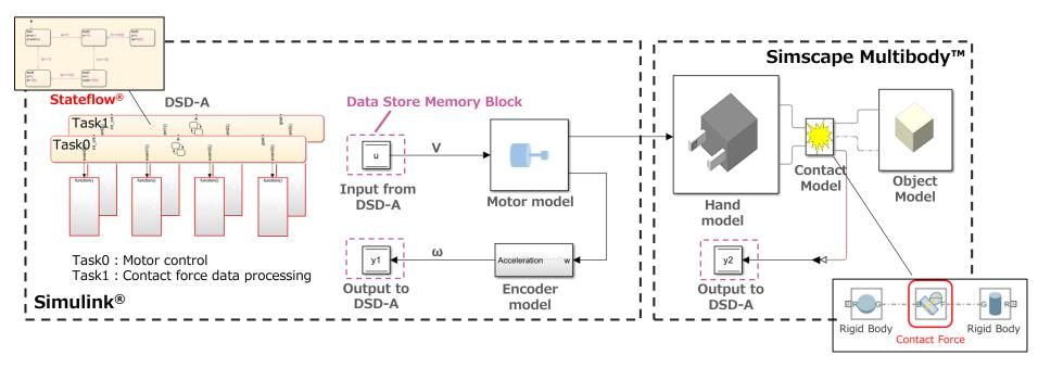
+ The robot hand components drawn in the block diagram are modeled by Simulink<sup>®</sup> and Simscape<sup>™</sup> Multibody<sup>™</sup>.
