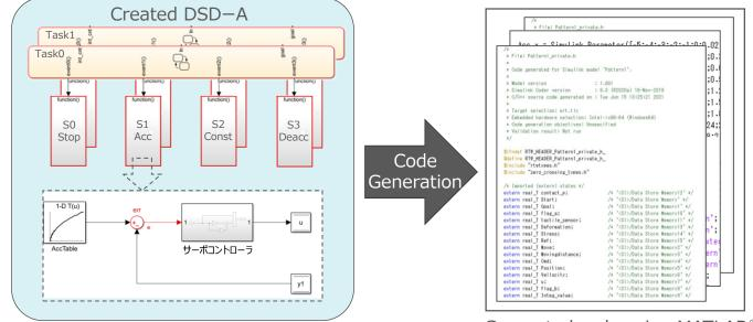
Generated code using MATLAB<sup>®</sup> Embedded Coder
