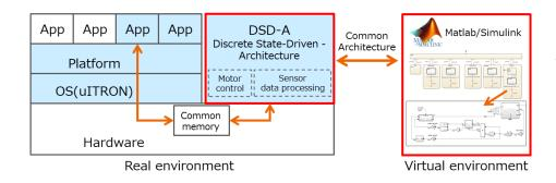
+ DSD-A part can be described by Simulink and has a common architecture in real and virtual environments.
