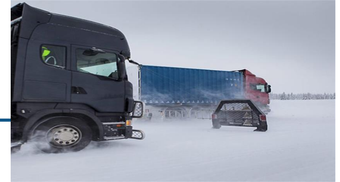
A controlled road test of Scania's advanced emergency braking system software.
