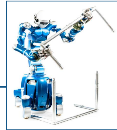
DLR's humanoid robot Agile Justin autonomously performing a complex construction task.
